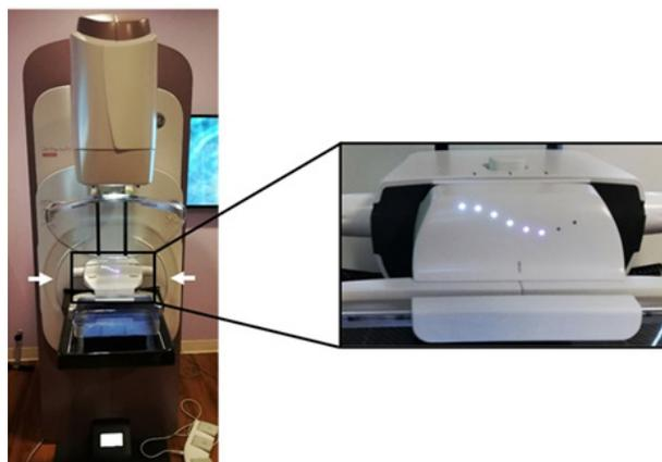
**Figure 1.** Research version of a flexible pressure-based compression paddle which is easily fitted to a Senographe Pristina DBT system (GE Healthcare, Chicago, IL). Eight light emitting diode (LED) lights indicate the pressure level to the technologist and participant. LED lights #5–7 (pink) indicate the target pressure range (8–13.9 kPa)
